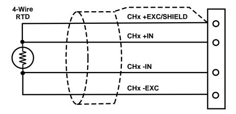
Figure 5: MAQ20-RTD41 4-Wire RTD Sensor Wiring
