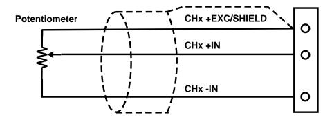
Figure 3: MAQ20-RTD31 Potentiometer Sensor Wiring
