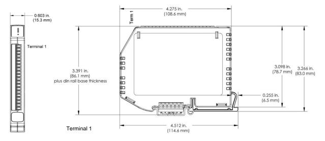
Figure 1: Module Dimensions
