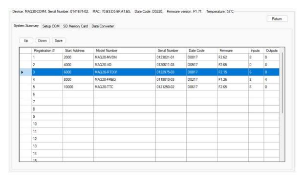
Figure 10: Viewing and Changing Module Registration using MAQ20-940 ReDAQ Shape for MAQ20
