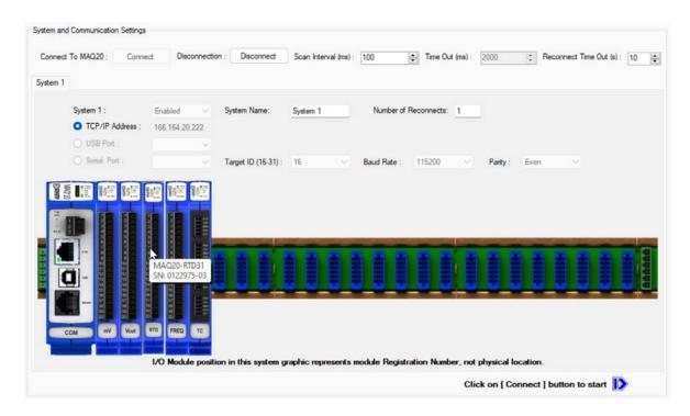
Figure 9: MAQ20-940 ReDAQ Shape for MAQ20 Main Configuration Screen with Graphical System Representation
