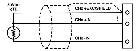
NOTE: Jumper +EXC to +IN for 2-wire sensors.
