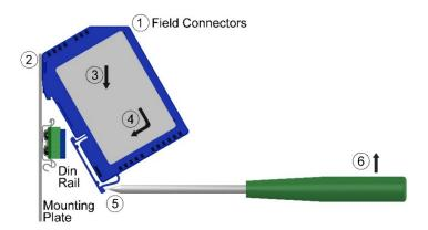
Figure 6: Module Installation and Removal
