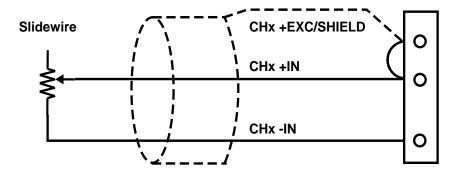
Figure 4: MAQ20-RTD31 Slidewire Sensor Wiring
